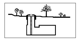
1. **Bunkers** are primarily underground shelters for protection against direct fire weapons and artillery. Bunkers have complete overhead cover and lack firing slits and embrasures. They are not meant to be fighting positions. Bunkers usually only have one entrance, which may be separate and linked to the bunker by a corridor or tunnel. Some bunkers are built above ground, but these are always heavily armored.
